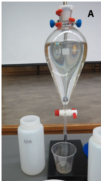
Figure 1: A) Separatory funnel, and B) filtration apparatus for microplastics filtration.
