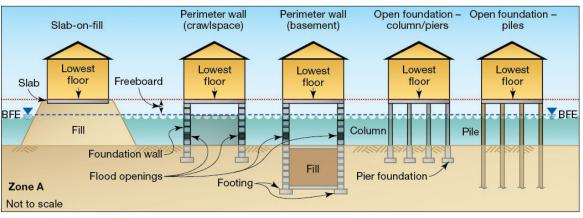
Structures elevated on posts, piles or piers as well as infilling basement up to ground level. (FEMA)
